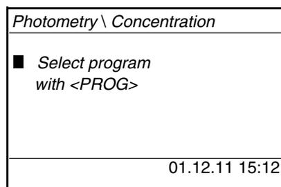
Using **<M>**, switch between the measured parameters *Concentration*, *Absorbance* and *% Transmission*.
