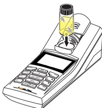
**Inserting a 16 mm cell**
